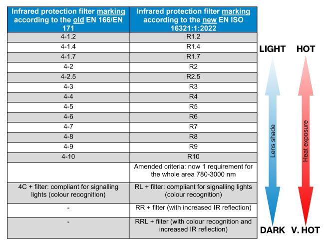
Signal recognition remains an optional test under the EN ISO 16321:1:2022 (as it did under EN171) however, it is depicted by an L if it meets the standard (instead of a C)
